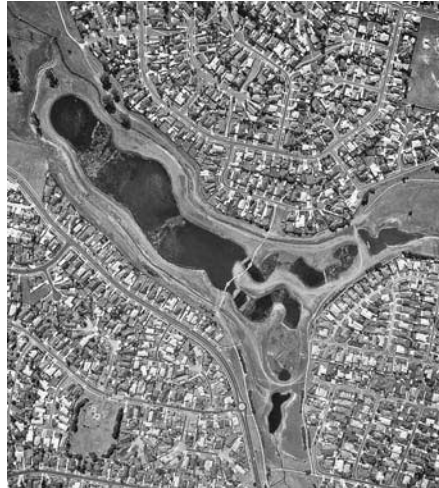
Figure 7.3 Constructed wetland for stormwater treatment at the regional scale (Melbourne).
