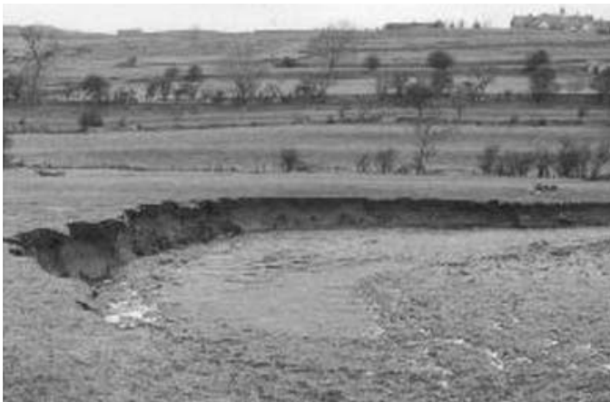
Figure 6.5: The Reeth monitoring site mid-catchment on the River Swale (15 January 1997). The 2 m high bank was modified by slab, pop-out and cantilever block failures. Flow is into the page.
