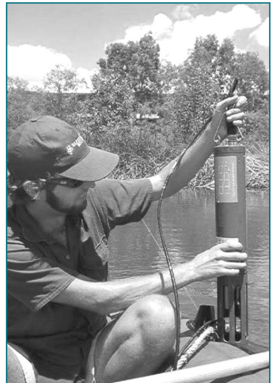
Figure 8.1 Boating at Bridgewater Creek Wetland - insitu measurement of water chemistry parameters
