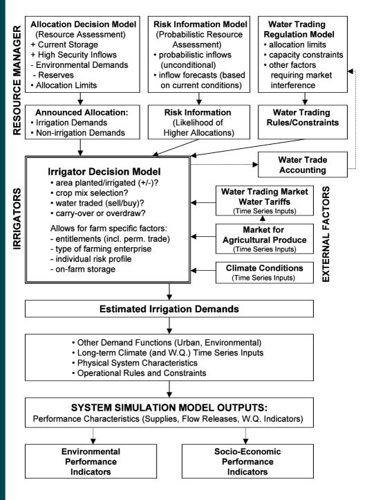
Figure C: Overview of water resource system simulation process, with emphasis on modelling irrigation demands
