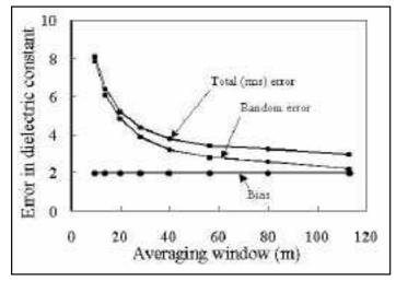
Figure B: Errors in dielectric constant (effectively soil moisture) estimation using L band AirSAR images at Tarrawarra on 11 November 1996.
