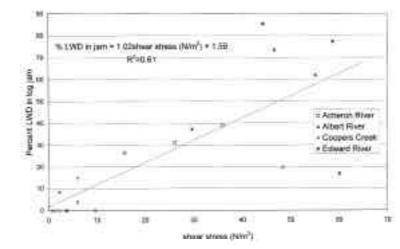
Figure D: Proportion of LWD in jams as a function of reach average shear stress.
