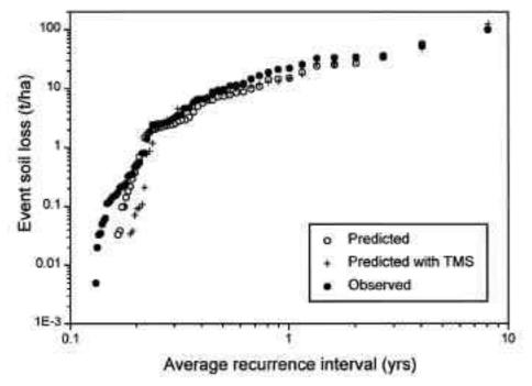
Figure A: Predicted and measured soil losses
