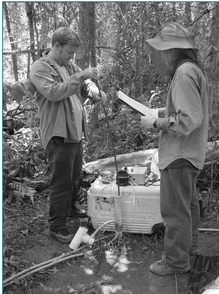
Figure 2.2: Christy Fellows and Andrew Mullens conducting a tracer study using the 'push-pull' technique to measure denitrification in the field.
