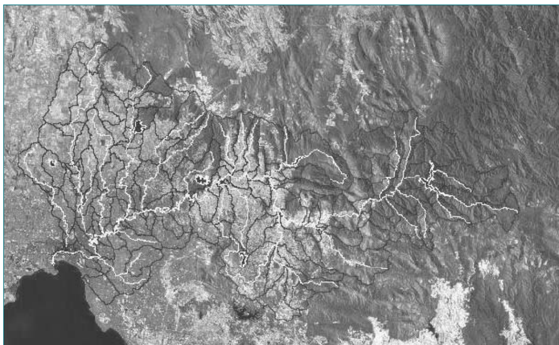
Figure 5.3, The YarraSim model is taking shape. Yarra Sim now incorporates a digital elevation model, a satellite image overlay, successful stream routing and rainfall fields that are being calibrated
