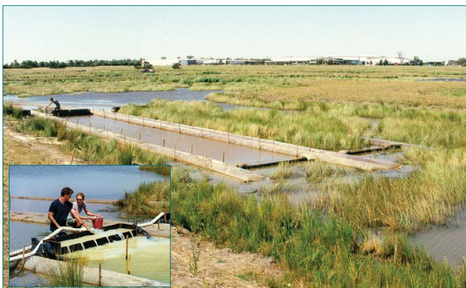
Figure 4.2. Testing the applicability of the k-C* algorithm using field dosing tests in Hallam Valley Wetland, Victoria.
