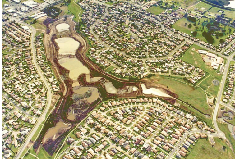
Plate 14. Hampton Park wetlands installed to reduce nutrient runoff to Port Phillip Bay (Photo courtesy Melbourne Water)
