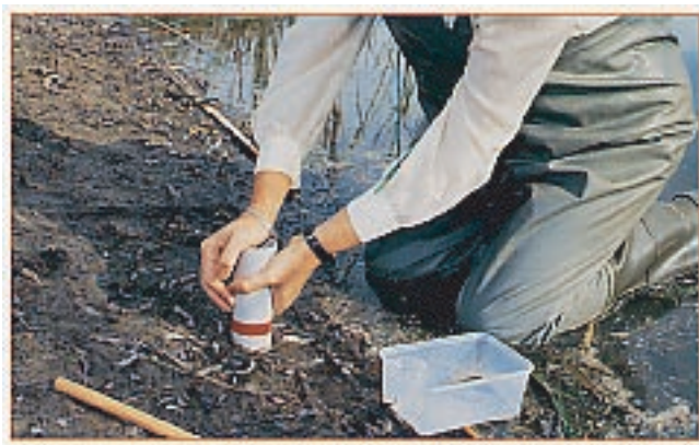
Taking a soil core with the corer.
