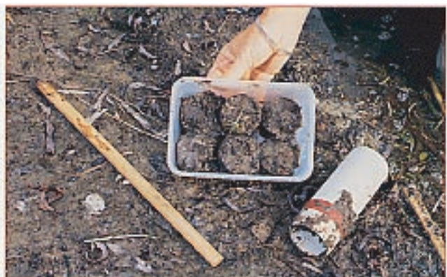
Soil cores, top side up, ready for drying.
