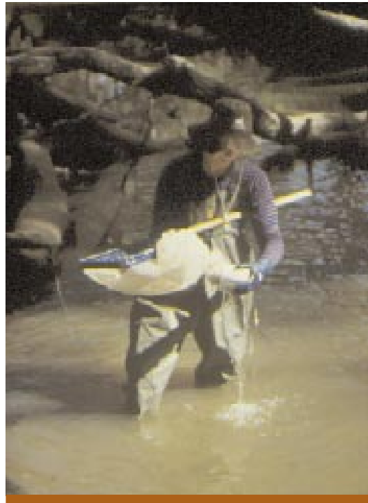
Jane Growns uses the 'snag bag' she developed to sample macroinvertebrates on snags in the Campaspe River. Photo: MDFRC
