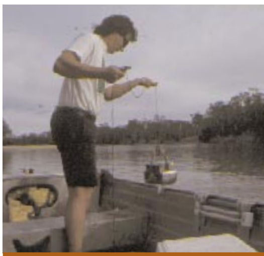
Ben Gawne sampling bottom-dwelling invertebrates using an 'Eckman Grab' on the River Murray. Photo: Lower Basin Laboratory
