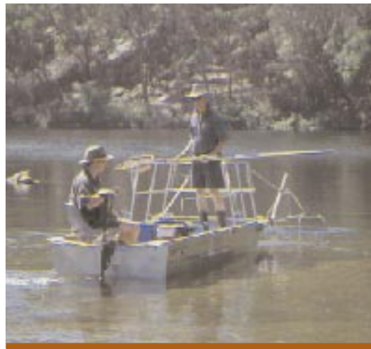
NSW Fisheries staff launched a new compact, lightweight electrofishing punt, Polt Volt , in the Woronora River early this year. The punt is designed to sample fish in small habitats. Photo: Rossana Silveira
