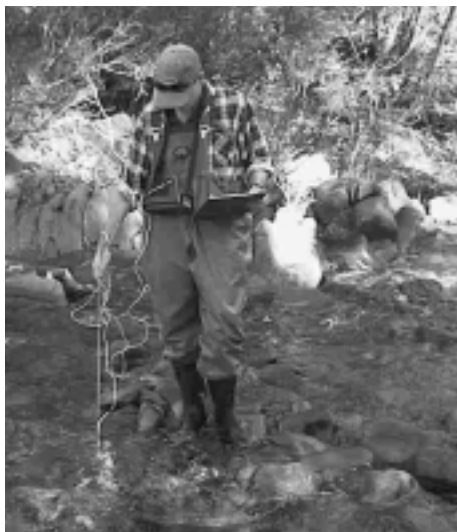
Measuring stream velocity using a flow meter for the First National Assessment of River Health.
