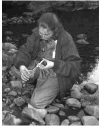
Nerida Davies calculating alkalinity for assessing river health using the AUSRIVAS model. Photo: P Sloane
