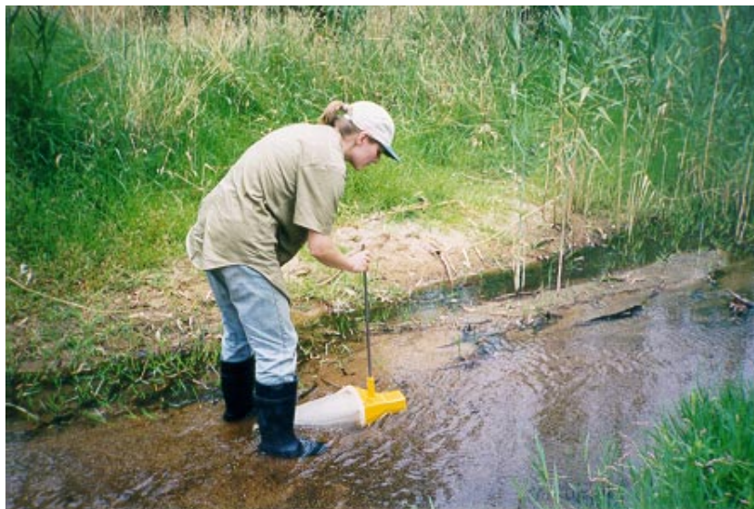
Fig. 3.7. A small Helley-Smith Bedload Sampler being used to sample bed load in Creightons Creek
