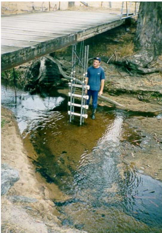
Fig. 3.6. Two views of the suspended sediment sampler
