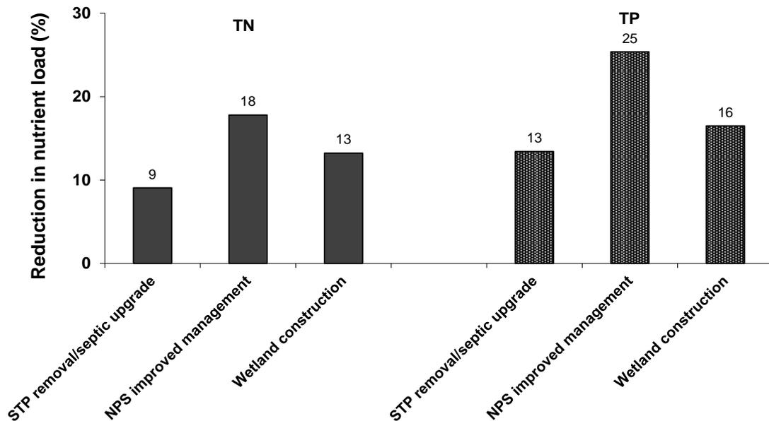
**Figure 4:** Modelled TN and TP estimates of load reductions to Lake Tai as a result of implementing three different improved practices: point source management, non-point source management and wetland construction.
