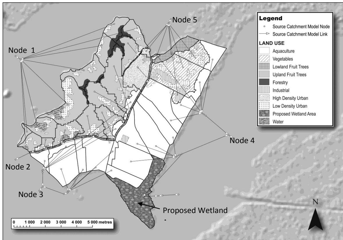
**Figure 2:** Source Landuse and subcatchment configuration with the node link network overlaid.
